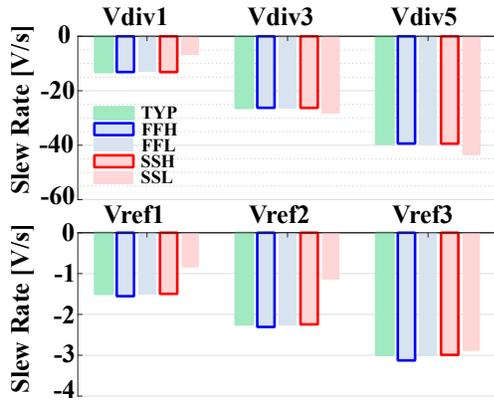
Fig. 8. Slew-rates of the divider (top) and reference (bottom) levels across five relevant corners.
