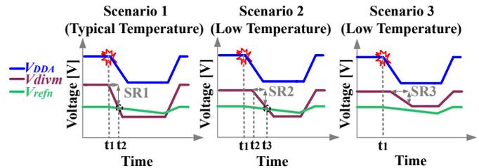
Fig. 1. Low-temperature impact on voltage-divider slew-rate.
