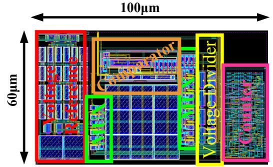
Fig. 6. BOD cell layout view.
