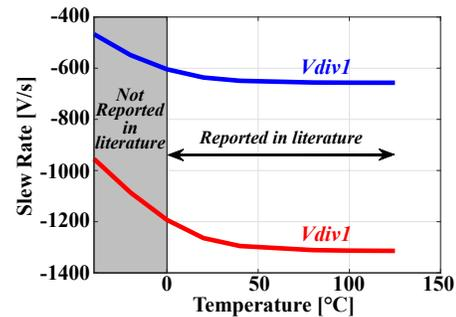
Fig. 3. Slew-rate vs temperature at voltage-divider.
