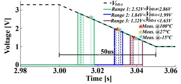
Fig. 7. BOD signal transient measurements and simulations for a supply voltage slew-rate of  $-46\text{V/s}$  during 50ms and PT variations.
