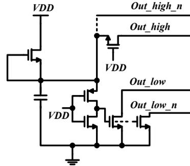
(b) BOD for pull-down and pull-up internal POR nodes [5].
