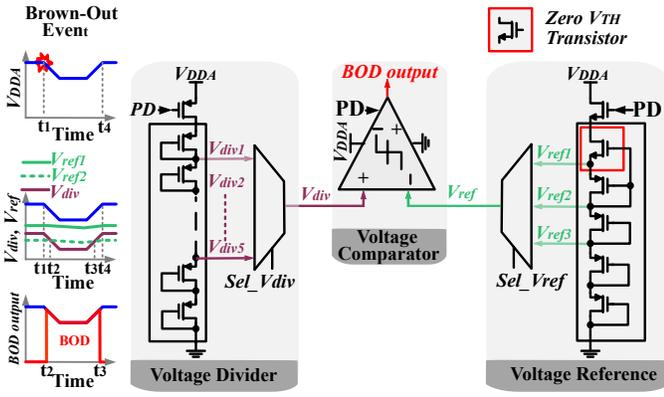
Fig. 4. Proposed BOD block diagram highlighting the proposed voltage divider and voltage reference schemes.
