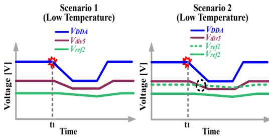
Fig. 5. Low-temperature trimming compensation for brown-out detection.
