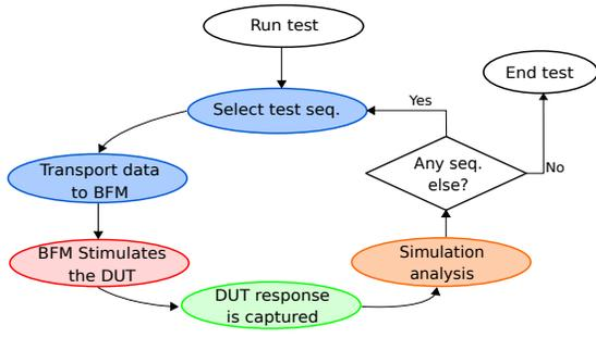
Fig. 2. Execution steps of a UVM-based VIP .
