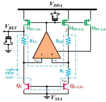
Fig. 6. Bandgap voltage reference schematic.
