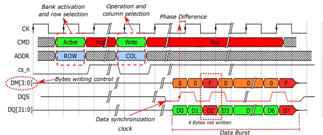
Fig. 1. LPDDR3 data transferring protocol.
