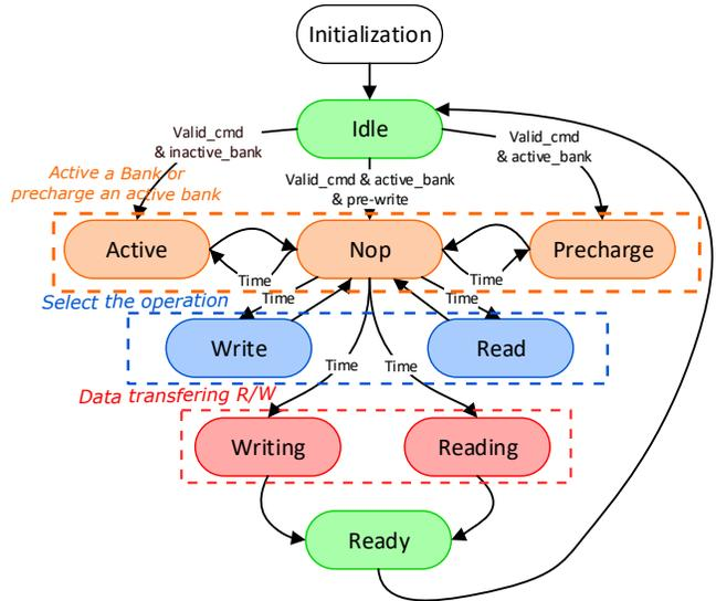
Fig. 3. State machine of the memory interface adapted as BFM.
