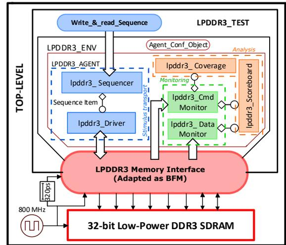
Fig. 4. UVM-based VIP diagram blocks for LPDDR3 memory.
