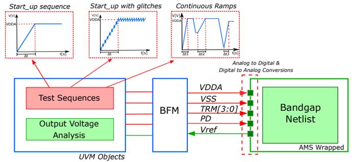
Fig. 7. Bandgap VIP diagram blocks.
