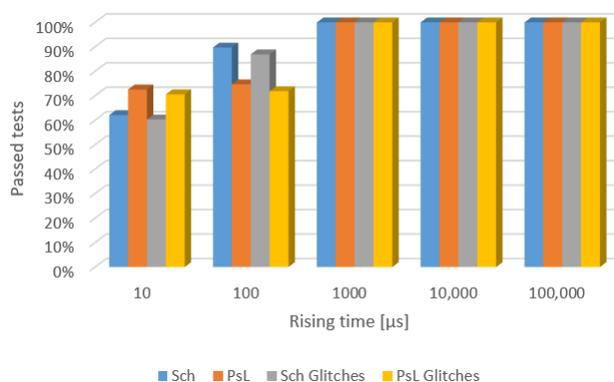
Fig. 8. Bandgap simulation results for start-up ramps tests.
