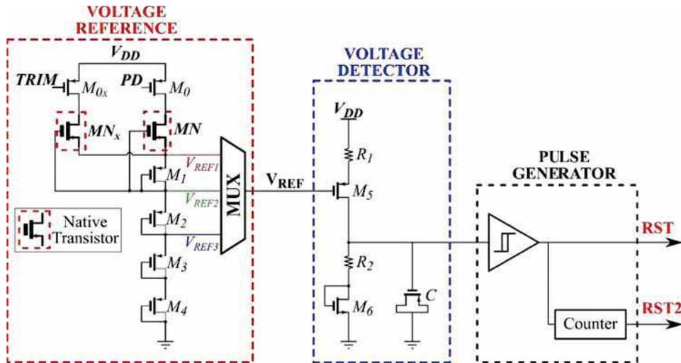
Fig. 3: Proposed POR circuit.
