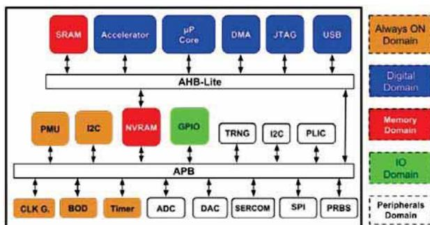
Fig. 2: Microarchitecture details of the SoC with clearly identified voltage domains.
