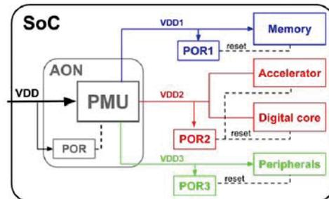
Fig. 1: SoC with multiple supply voltage domains.
