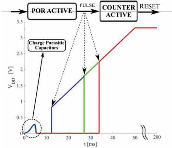
Fig. 5: POR Signal for a  $V_{DD}$  ramp of 50ms.
