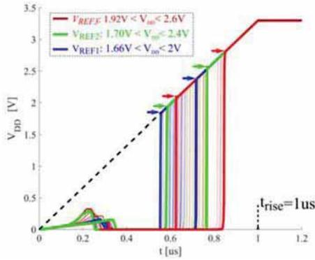
Fig. 6: POR signals corners case without trimming for  $V_{DD}$  ramp of 1us.
