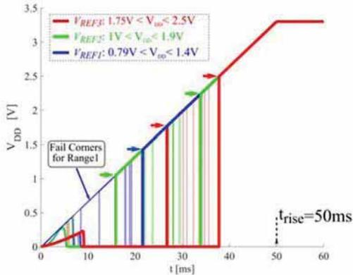
Fig. 7: POR Signals corners case without trimming for a  $V_{DD}$  ramp of 50ms.
