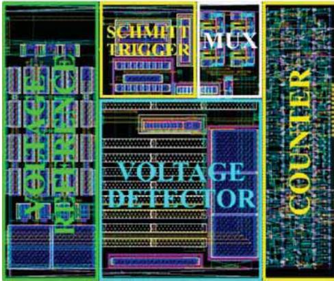
Fig. 4: Layout of the POR Proposed.
