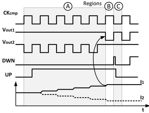
Fig. 2: Timing diagram of the offset-reduction technique.
