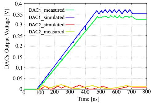
Fig. 8: Measured and simulated (TT) output voltage of calibration DACs during a calibration process.
