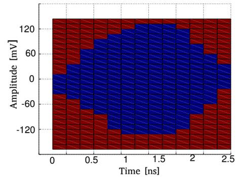
Fig. 10: Measured on-chip eye diagram after calibration.
