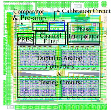
Fig. 5: Layout of the circuit that includes the proposed offset-correction technique.
