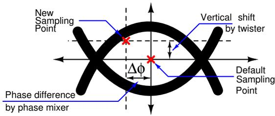
Fig. 6: Conceptual diagram of phase and voltage shifting to build the eye-diagram at the pre-amplifier input.
