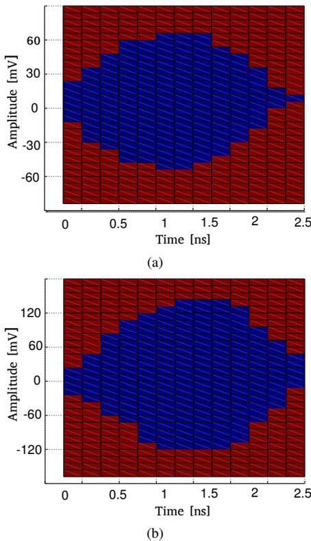
Fig. 9: Measured on-chip eye diagram before calibration: a) with 21dB of attenuation, b) with 14dB of attenuation.
