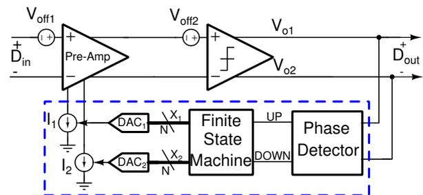
Fig. 1: Block diagram of the proposed offset reduction technique.
