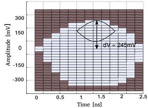
Fig. 11: Maximum unbalance range that the calibration can compensate.
