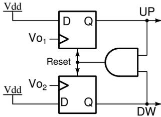
Fig. 3: Phase and frequency detector.
